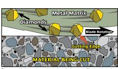
The exposed diamond crystals do the grinding work. The metal matrix or bond holds the diamond in place. Trailing behind each exposed diamond is a bond tail which helps to support the diamond. As the blade rotates through the material, the exposed surface diamonds grind the material
